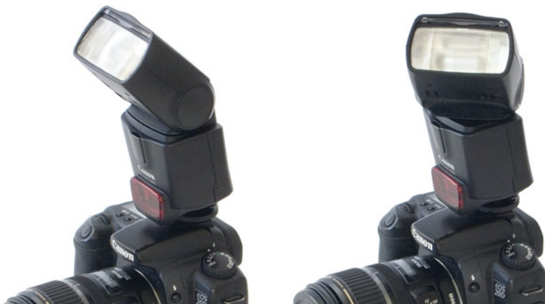
FIGURE 9.8 A flash unit that can tilt and swivel offers many more options for creating flash shots with natural-looking lighting.
